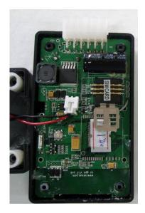
3 Put the SIM card into the holder, and turn the foil right and fasten it in place.
